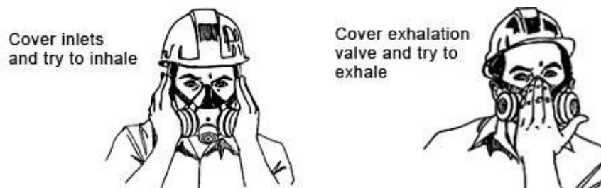
Figure 5.2: Inspection of respirator to ensure proper seal. No leakage should occur. (Left) – Negative pressure check. (Right) – Positive pressure check.
